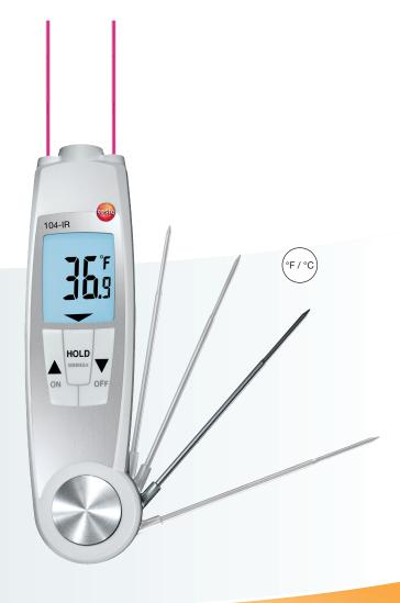
The testo 104-IR is a waterproof (IP65) penetration thermometer combined with an infrared sensor for non-contact temperature measurement. It can be used for various applications in the food sector. The precise testo 104-IR scans the surface temperature of individual foods or entire pallets from a distance. If a limit value is exceeded or undershot, the hinged penetration probe is also able to measure the core temperature.
